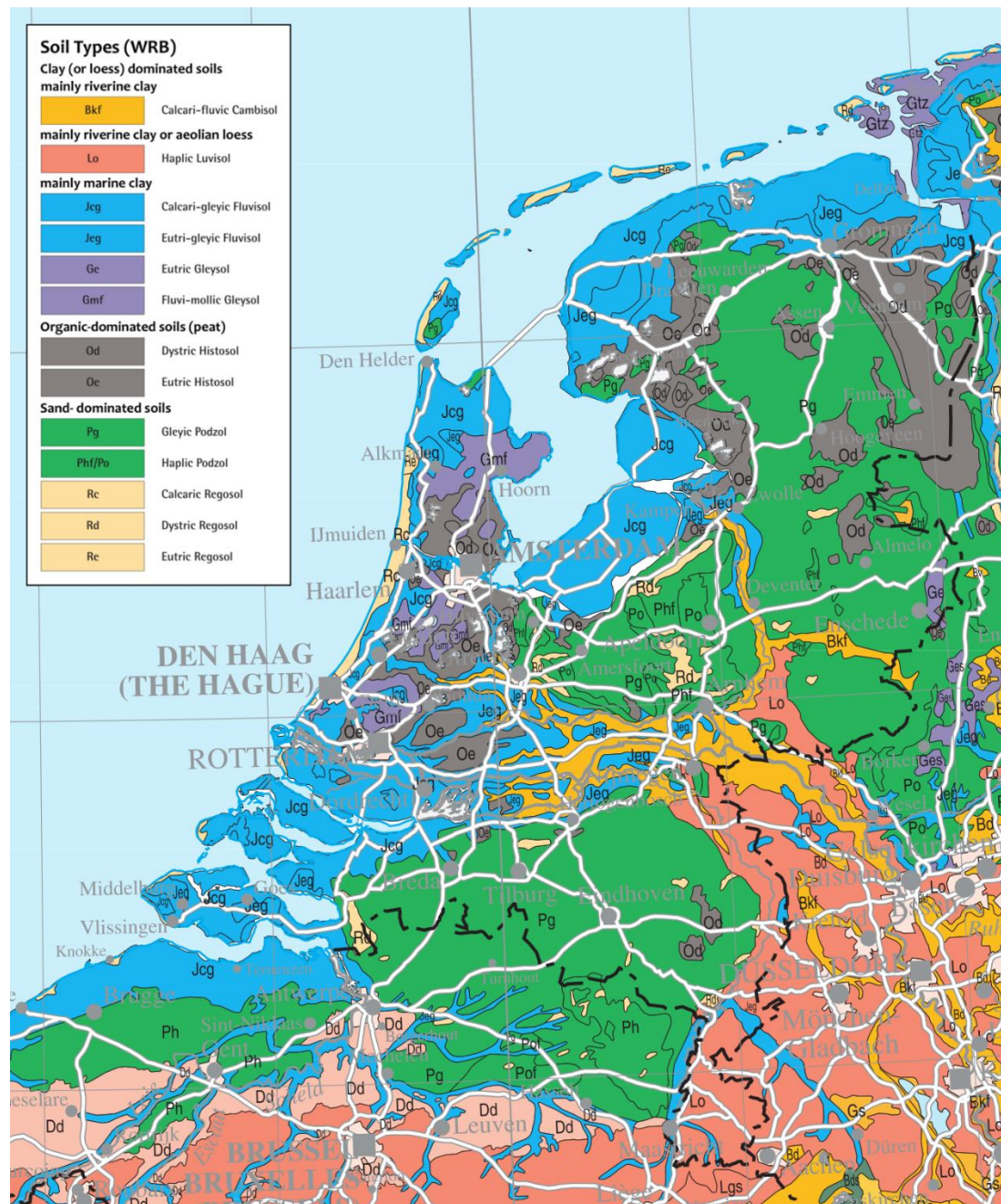
Figure 5: Main soil types in the Netherlands (World Reference Base), grouped approximately according to dominant texture. Source: Soil Atlas of Europe, 2005 2 .
