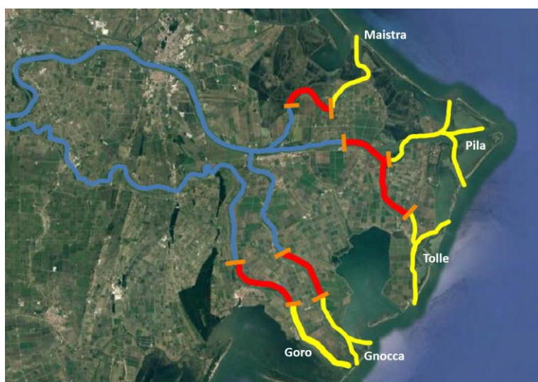
Figure 11: Sea water intrusion distance in km on 16 th March 2022 compared to the summer values observed in 2003 (upper) and location of river branches (lower). Source: Permanent Observatory on water use - Po River District Basin Authority.
